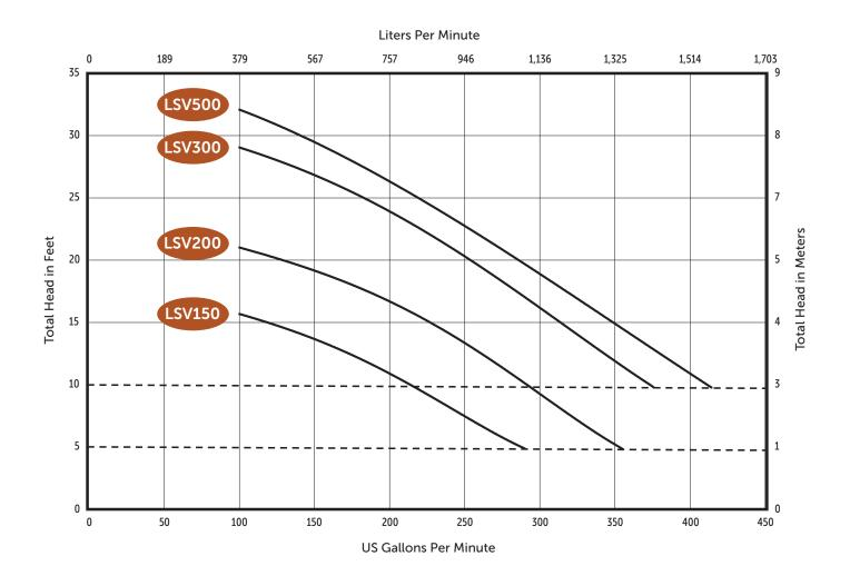
LSV150 and LSV200 Series models have a 5 ft. minimum head requirement.
